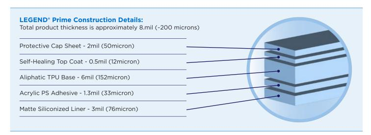
**LEGEND® Self-Leveling Hydrophobic surface** is formulated for long-lasting gloss retention. The minor scratches and mars caused by normal wear, such as car wash, are seamlessly eliminated over time. Our low surface energy of the topcoat prevents surface darkening caused by water-borne contamination. The car surface with LEGEND® Paint Protection Film installed retains attractive smooth high-gloss appearance for years to come maintenance free.
