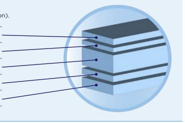
**LEGEND® Select Fast Self-Healing Top Coat** is formulated for a long-lasting, quick rebound from minor damage such as car wash scratches and scuffs caused by regular driving. Car surface with LEGEND® Select Paint Protection Film installed retains attractive smooth high-gloss appearance for years to come maintenance free.
