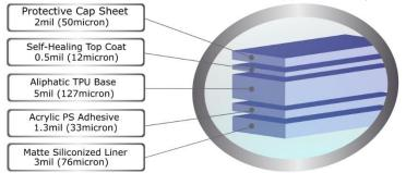
**LEGEND® Select Fast Self-Healing Top Coat** is formulated for a long-lasting, quick rebound from minor damage such as car wash scratches and scuffs caused by regular driving. Car surface with LEGEND® Select Paint Protection Film installed retains attractive smooth high-gloss appearance for years to come maintenance free.
